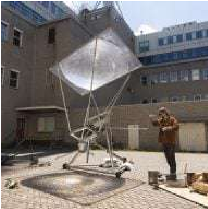
Solar Metal Smelter uses giant magnifying glass to melt metal
